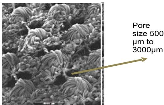
**Figure 17** Embroidered textile structure with pore size 500µm to 3000µm.
