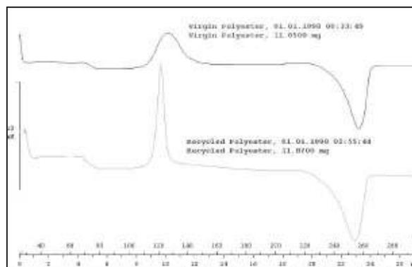
**Figure 7** Thermal graphs of virgin and recycled polyester fibres
