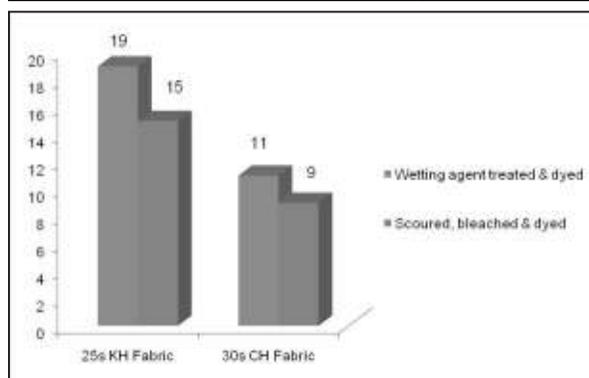
**Figure 9** Bar chart showing the average no. of neps per 10cm<sup>2</sup> of fabrics dyed through different process routes
