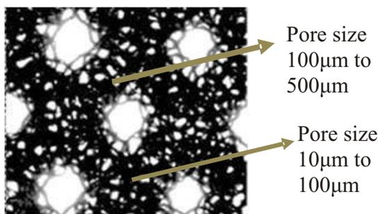
**Figure 16** Embroidered textile structure with pore size 10µm to 500µm.
