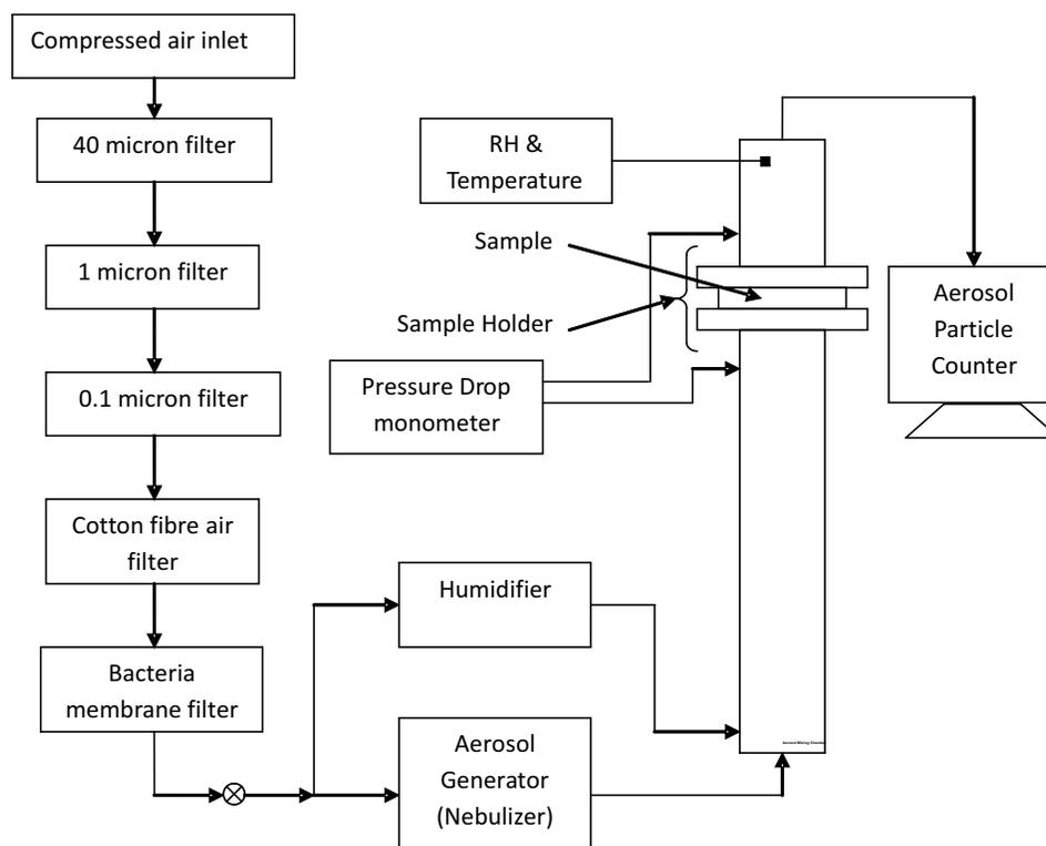
**Figure 23** Line diagram of Particle Filtration Efficiency Tester developed by SITRA
