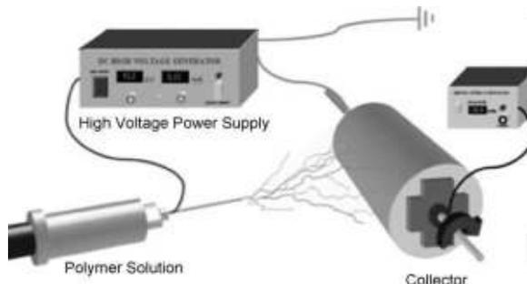
**Figure 21** Schematic representation of electro-spinning set-up
