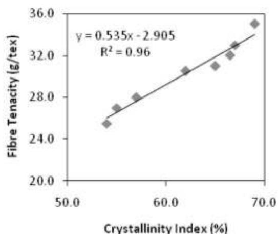
**Figure 1** Relationship between crystallinity Index and fibre tenacity
