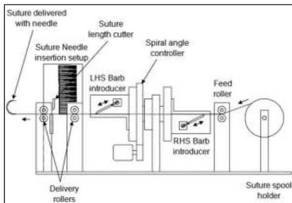
**Figure 22** Schematic diagram of SITRA's Knotless Suture Manufacturing Machine (SKSMM)
