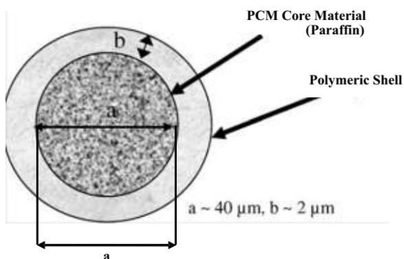
**Figure 10** PCM core material with a hard polymeric shell.
