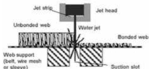
**Figure 20** Schematic representation on of Hydro-entanglement process
