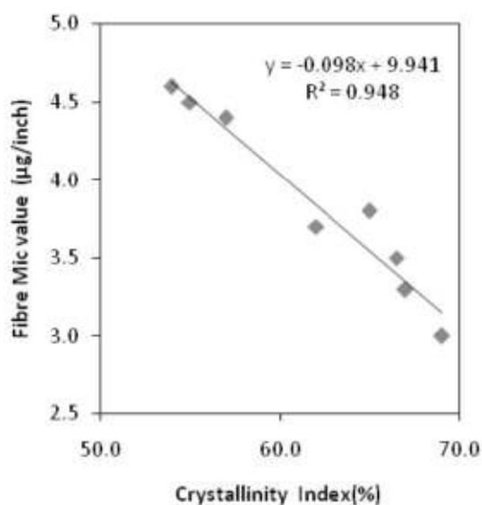
**Figure 2** Relationship between crystallinity index and fibre Mic value
